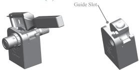
7. Press downward on handle-end of cartilage knife (B) to cut cartilage specimen into desired thickness. **IMPORTANT!** To avoid difficulty in removal of blade (A) from cartilage knife (B), do not use excessive force when pressing downward.
